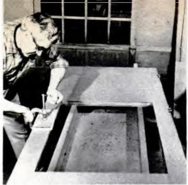
POSITION PANEL and drive a few brads to prevent it from shifting. Use weights until the glue is dry
